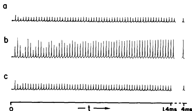
FIG. 5. The evolution of S magnetization ( S_x ) as a function of cross-polarization time t during a Hartmann-Hahn experiment for three different S spin rf field strengths, \omega_{1S}/2\pi \approx (a) 40 kHz, (b) 51 kHz, (c) 71.3 kHz. The I spin rf field was held constant at \omega_{1I}/2\pi \approx 54 kHz. The transient oscillations described by Müller et al. (Ref. 27) are prominent near Hartmann-Hahn match (b). The described polarization of the S spins in (a) and (c) is clearly not a result of competing cross-polarization and spin-lattice relaxation, as is usually claimed, because the signal remains constant over a considerable period of time. It must be explained instead by the establishment of a quasi-equilibrium state.
